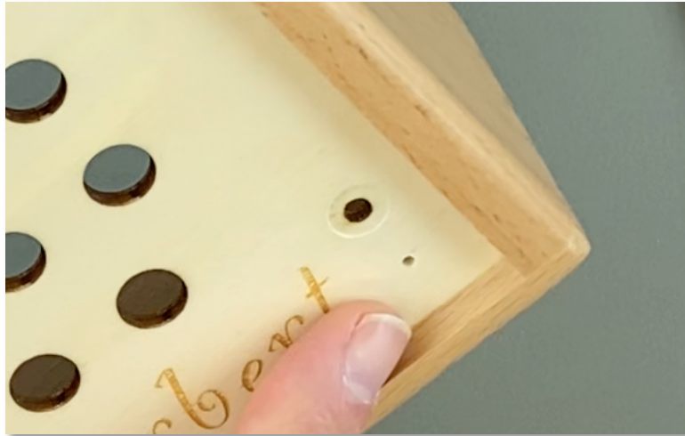
Figure 4 - Microphone LED Display Drill Hole
