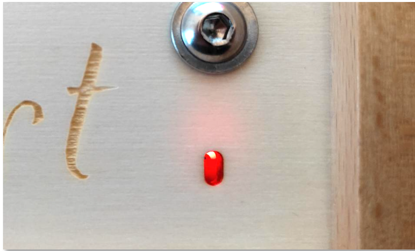
Figure 8 - Microphone LED Lights Up Red When Recording
