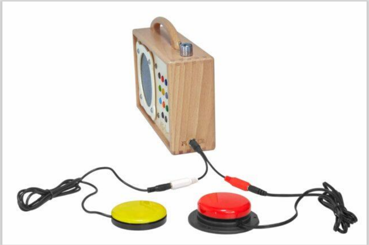
Figure 7 - hörbert connected with external control buttons via Y-cable
