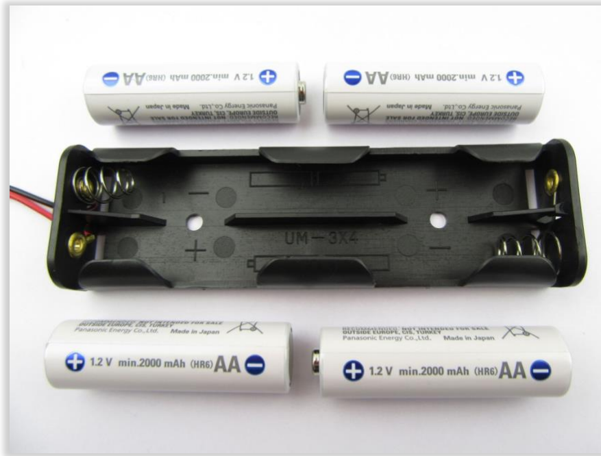
Figure 3 - Battery Charging Compartment - Polarization of the Batteries
