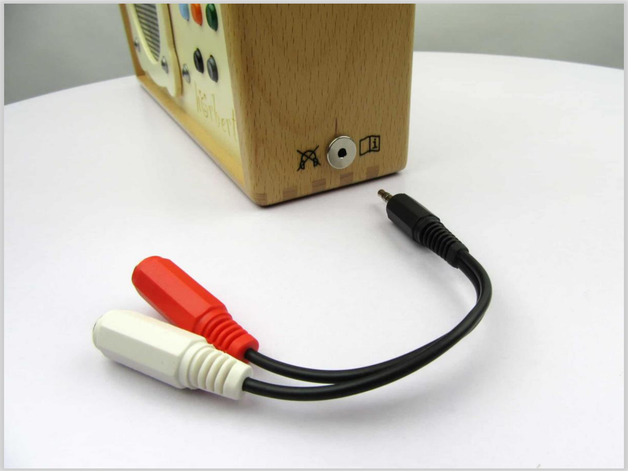
Figure 6 - Connection for external control button(s)
