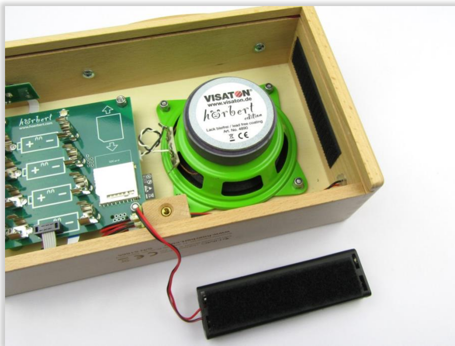
Figure 2 - hörbert with battery charging compartment - Velcro fastener
