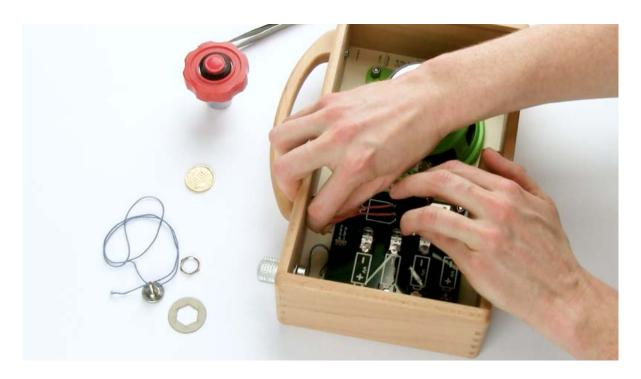
6. Disconnect the blue-white cable of the built-in volume control from the hörbert electronics in the same way. Leave the volume control screwed into the housing.
