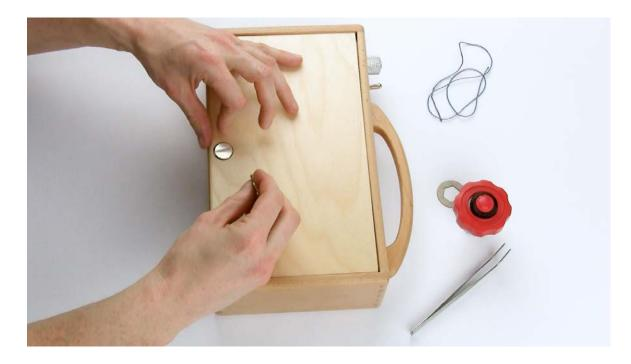
2. VERY IMPORTANT! Remove all batteries so that you do not accidentally destroy your hearing by a short circuit (from tools or jewellery). The thread that you run under a battery serves as an aid, in order to then pull it out. Repeat this for each battery individually.
