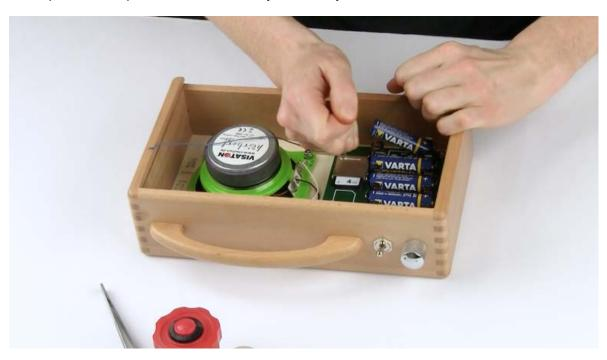
3. Place the cardboard washer over the existing nut of the on/off switch. It serves as a scratch protection when loosening the nut. Then use your tool to unscrew the nut counterclockwise.
