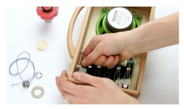
5. Pull the red cable of the switch out of the hörbert electronics. It provides some resistance until the plug clicks out. Do not tear upwards or downwards, but pull the plug straight out of the socket (in the direction of the cable).
