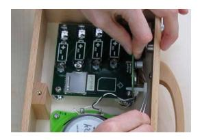
5. Now tighten the nut of the switch by hand using the scratch protection. Don't use too much force to keep the thread from tearing out.
