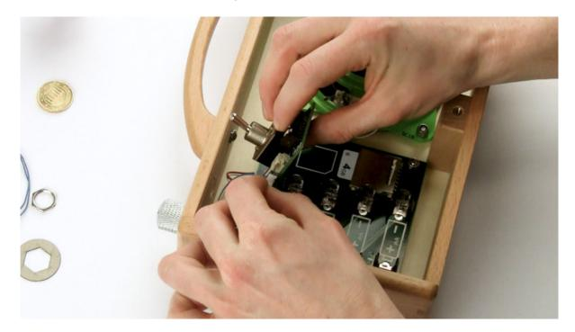
10. In the next step, guide the switch of the additional electronics back through the opening in the housing. The small white switches (the "mouse piano") point upwards, so that you can use it later comfortably.
