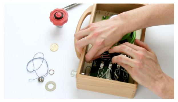
6. Now unplug the blue and white cable of the built-in volume control from hörbert's electronics in the same way. Leave the volume control screwed into the cabinet.
