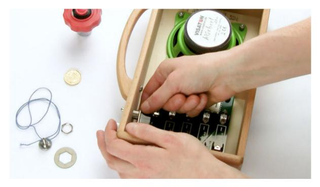
5. Pull the red cable of the switch out of the audio electronics. It offers some resistance until the plug clicks out. Do not tear upwards or downwards, but pull the plug straight out of the socket on the computer board.
