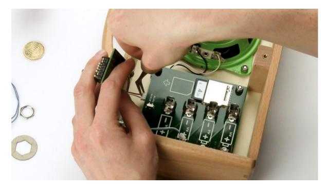
9. Finally, plug the remaining blue and white cable of the volume control into the free socket of the additional electronics. This completes the new cabling.
