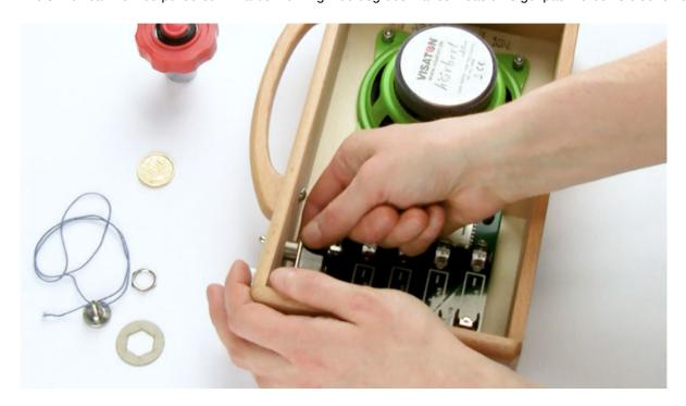
Pull the red cable of the switch out of the audio electronics. It offers some resistance until the plug clicks out. Do not tear upwards or downwards, but pull the plug straight out of the socket on the computer board.
