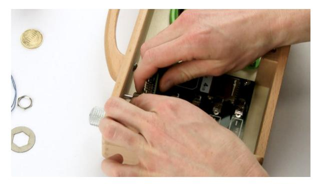
11. Tighten the nut of the switch again by hand. Do not use too much force to avoid tearing out the thread.
