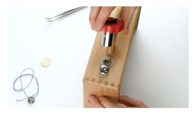
4. The switch can now be pulled out inwards. Turning it 90 degrees makes it easier to get past hörbert's electronics.
